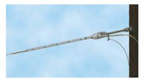
The FIBERLIGN® Formed Wire Dead-end has two spiral shaped wires comprising a structural rod on the inner layer and a dead-end component on the outer layer.
