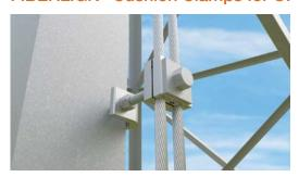
The FIBERLIGN® Downlead Cushion Clamps secure OPGW and ADSS cable downleads to structures while minimising compressive clamping forces that could transfer to the optical elements.
